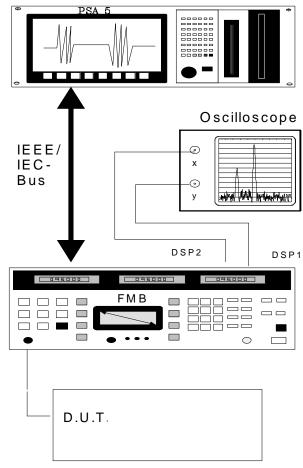
Fig.4. Test set-up for automatic test routine
