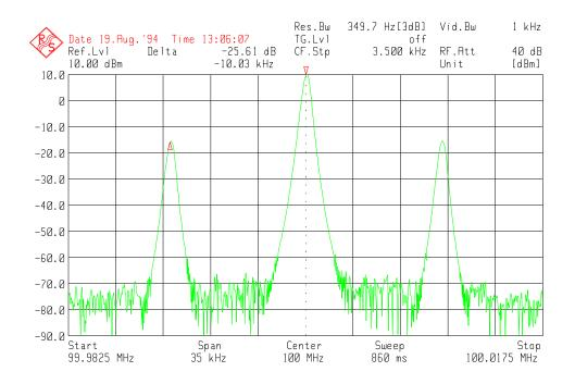
Fig. 2: The RF spectrum of the reference signal shows a sideband level of 26 dB
