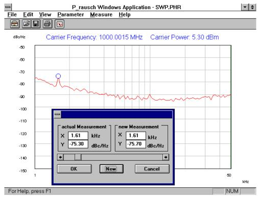
Fig. 7: Result of a repeated measurement using the Marker function
