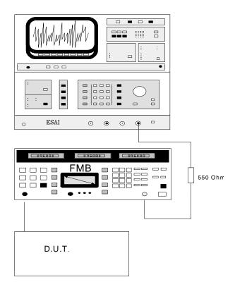
Fig. 1: Test setup with external spectrum analyzer
