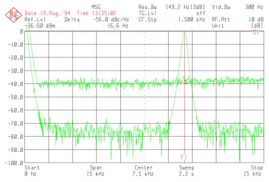
Fig. 3: The level of the demodulated reference signal is used as a reference (lines F1 and D1) in the phase noise measurement. The value of -56 dBc/Hz measured here must be corrected by 26 dB to allow for the carrier offset so that, as a final value, -82 dBc/Hz is obtained.
